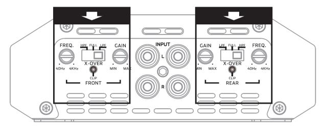
A crossover is a device that removes unwanted frequencies from a speaker or amplifier. A tweeter can easily be destroyed by bass notes if they are not filtered out. Likewise, a subwoofer will not sound natural if it is playing midrange notes. A crossover removes these sounds from the speaker. Careful adjustment is needed to ensure that all the speakers are playing the right sounds and that you are left with no "holes" or gaps in the frequency response.
