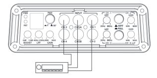
Connect your RCAs from the head unit to the RCA inputs on the amplifier.
