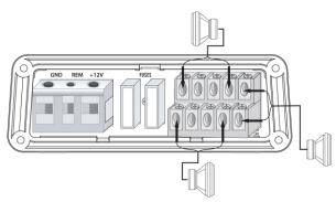
In bridged operation, connect the speaker wires as shown with an impedance of 4 Ohms or greater. The subwoofer channel must be 2 Ohms or greater.
