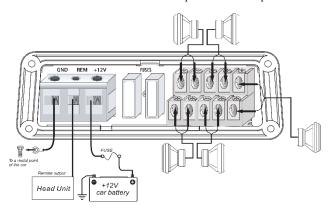
Connect the power wires and speaker wires as indicated. Use an impedance of 2 Ohms or greater.
